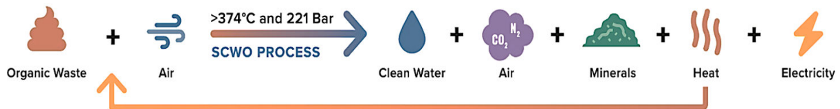
Figure 3. Supercritical water oxidation with AirSCWO™. Credit: 374Water.
