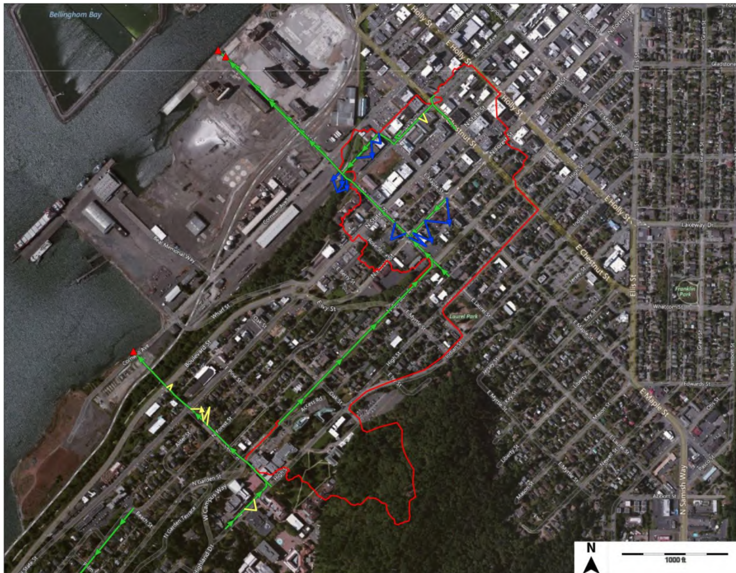
Figure A7. Schematic diagram showing the Laurel drainage network (green), active overflow paths (blue), and inactive overflow paths (yellow) during the 25-year flood event under full build-out land-use conditions. Overflow path locations are intended to be schematic only and do not indicate actual flowpaths. Drainage boundary is shown in red. The two Laurel system outfalls are shown as red triangles.
