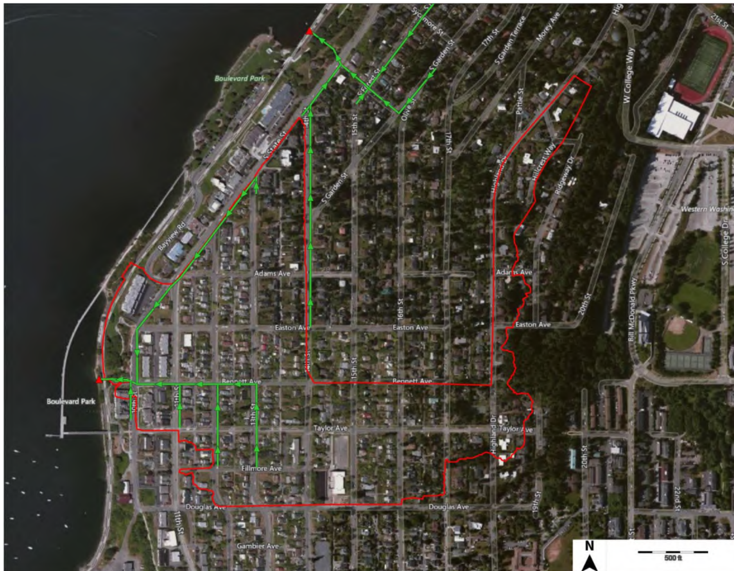
Figure A2. Schematic diagram showing the Bennett drainage network (green) during the 25-year flood event under full build-out land-use conditions. No overflow paths were identified in the Bennett system. Drainage boundary is shown in red. The Bennett system outfall is shown as a red triangle.
