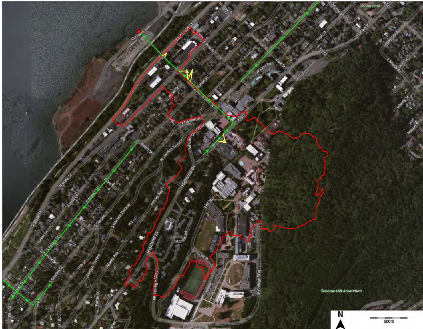
Figure A4. Schematic diagram showing the Cedar drainage network (green), active overflow paths (blue), and inactive overflow paths (yellow) during the 25-year flood event under full build-out land-use conditions. Overflow path locations are intended to be schematic only and do not indicate actual flowpaths. Drainage boundary is shown in red. The Cedar system outfall is shown as a red triangle.
