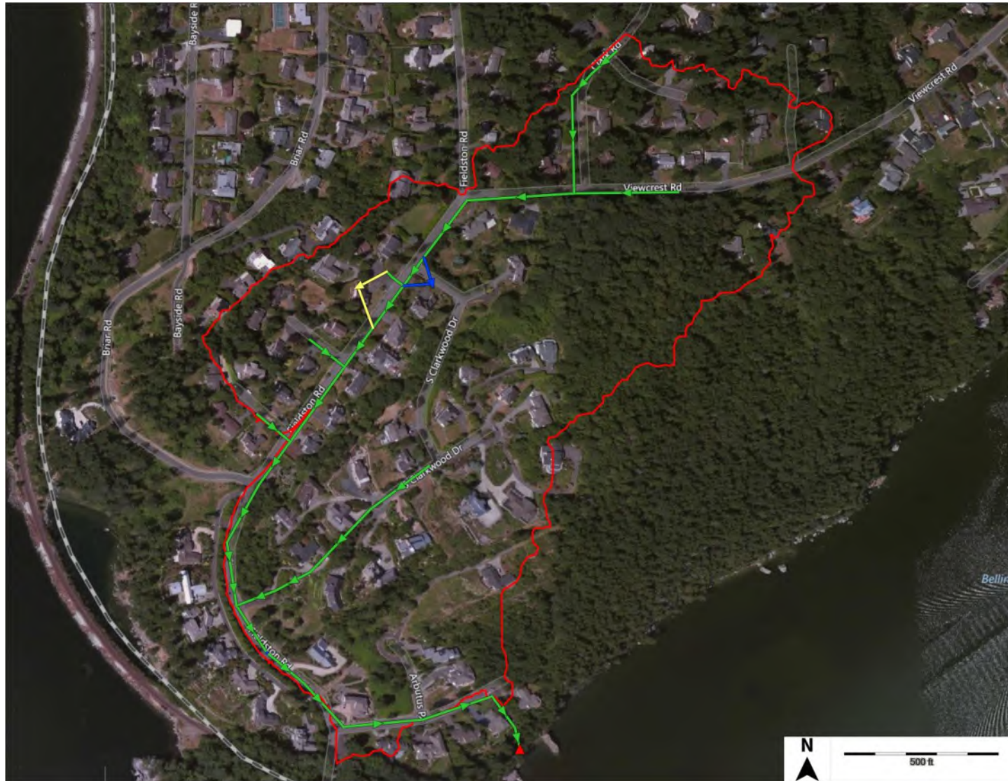
Figure A1. Schematic diagram showing the Arbutus drainage network (green), active overflow paths (blue), and inactive overflow paths (yellow) during the 25-year flood event under full build-out land-use conditions. Overflow path locations are intended to be schematic only and do not indicate actual flowpaths. Drainage boundary is shown in red. The Arbutus system outfall is shown as a red triangle.
