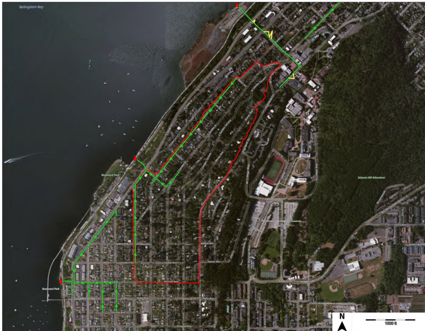
Figure A8. Schematic diagram showing the Olive drainage network (green) during the 25-year flood event under full build-out land-use conditions. The only overflow path identified in the Olive system is not shown; it is immediately upstream of the outfall. Drainage boundary is shown in red. The Olive system outfall is shown as a red triangle.
