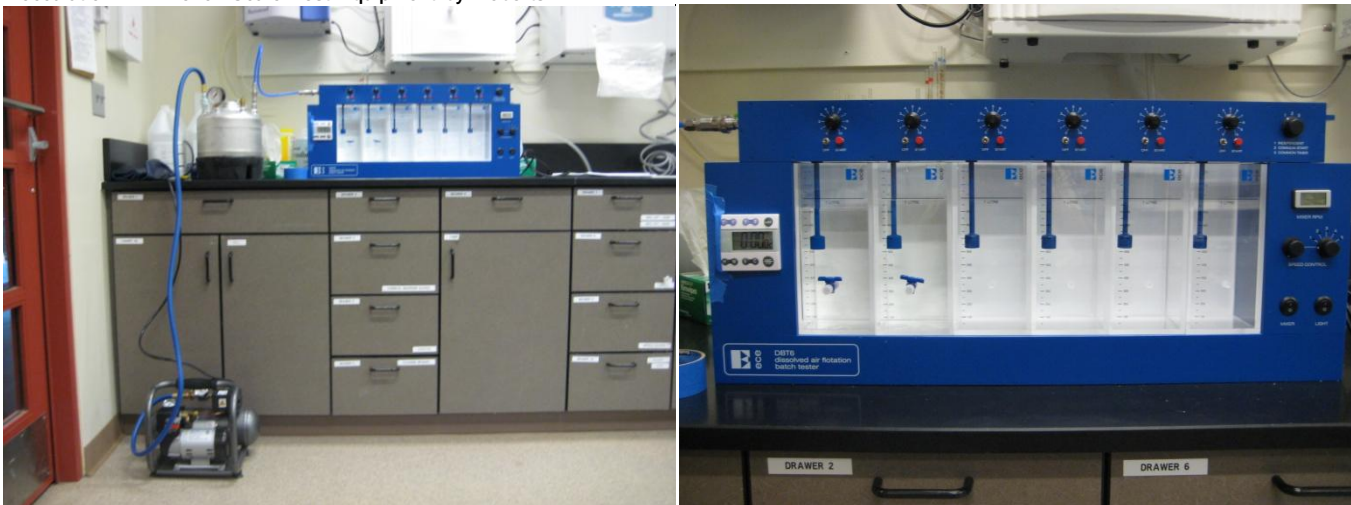
FIGURE 3-2 Flocculation/DAF Bench-Scale Test Equipment by Roberts
