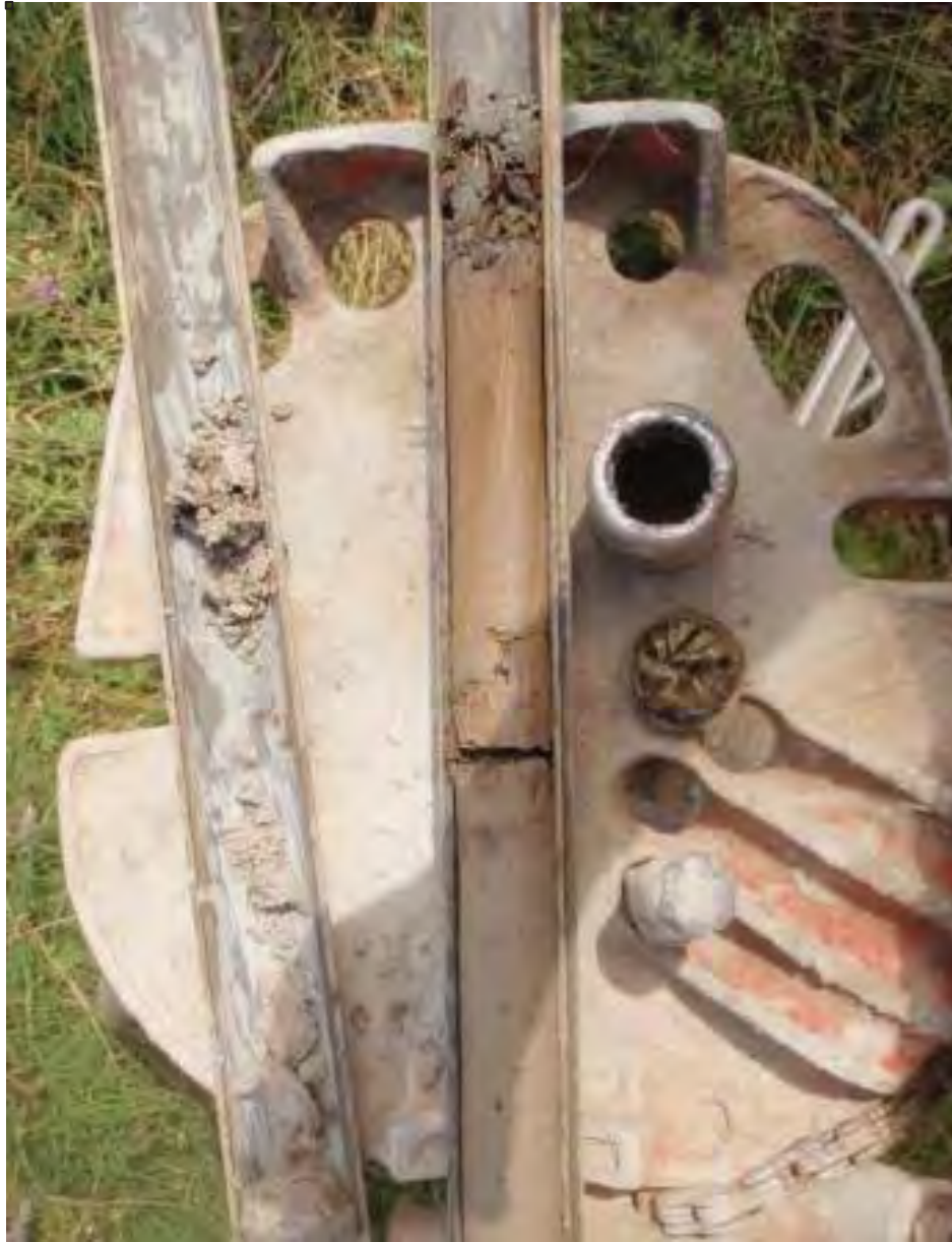
Figure 9. Geotest boring (B2) sample showing the upper sediments.
