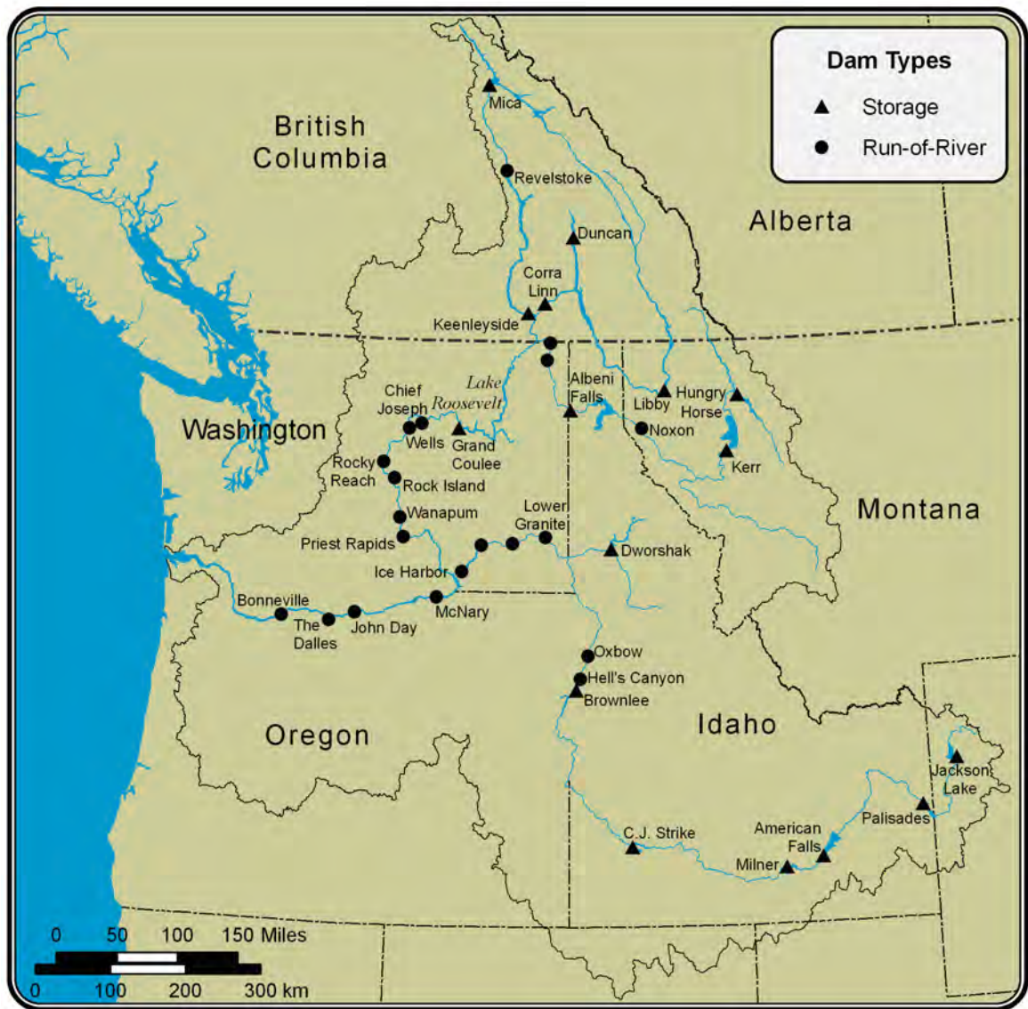
Figure 1. Columbia River basin projects incorporated in the ColSim reservoir model (note Snake River projects are aggregated in the model).
