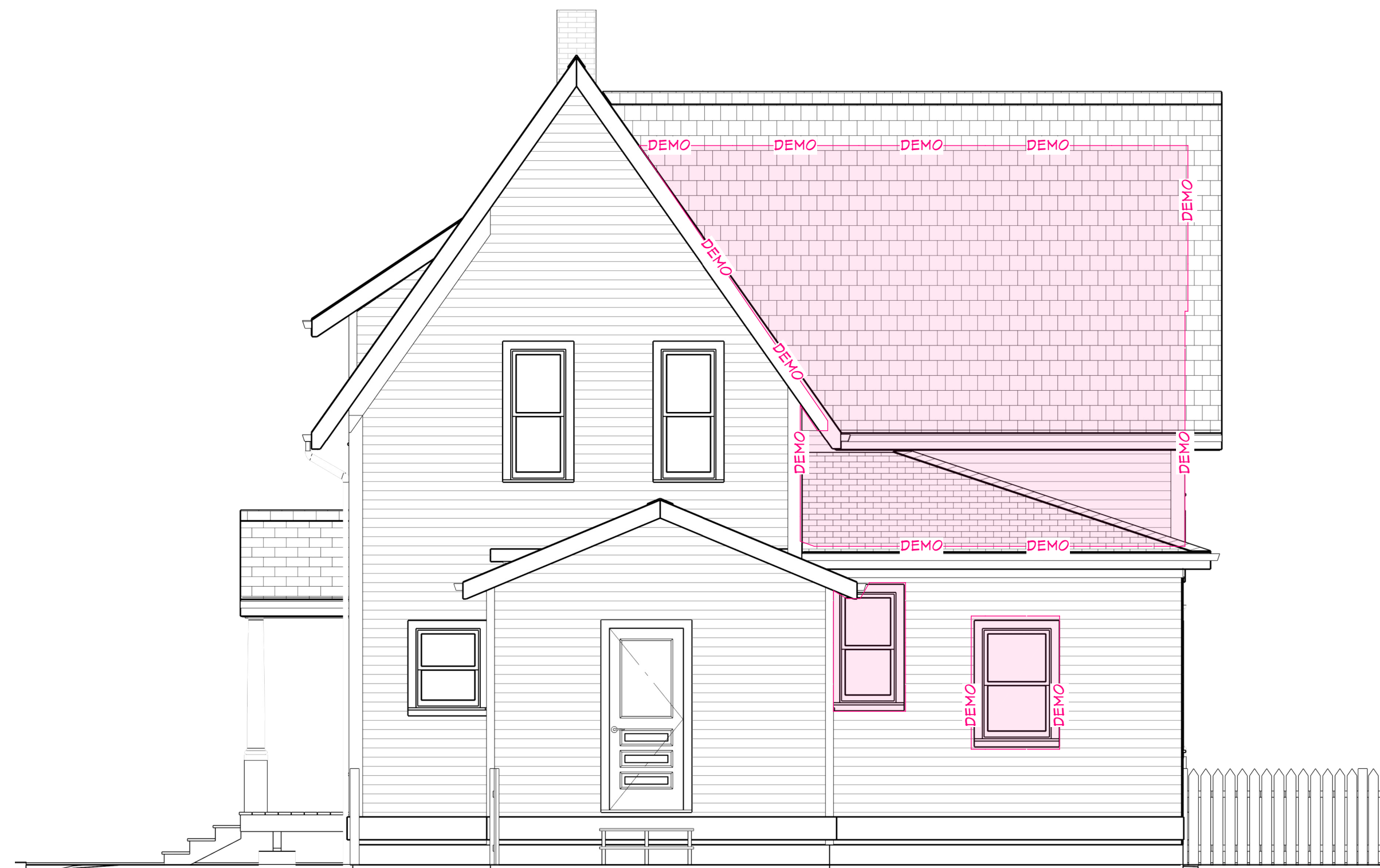
SOUTH ELEVATION EXISTING CONDITION / DEMO 1/4 in = 1 ft
