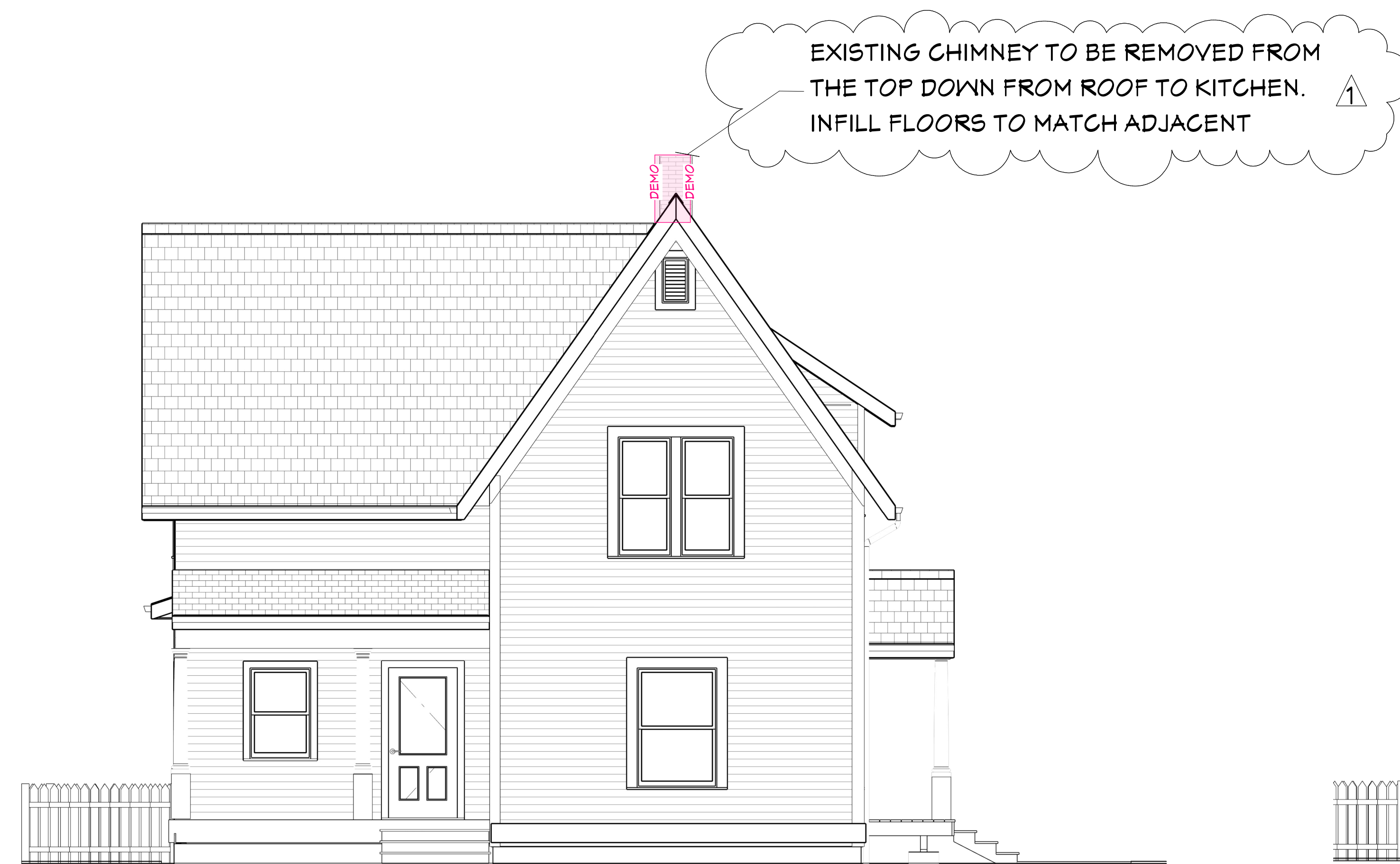
NORTH ELEVATION EXISTING CONDITION / DEMO 1/4 in = 1 ft
