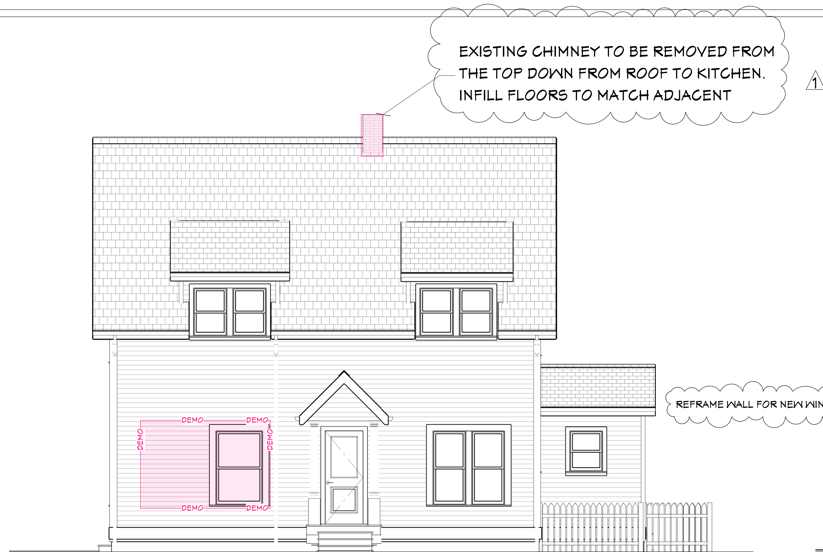
EAST ELEVATION EXISTING CONDITION / DEMO 1/4 in = 1 ft
