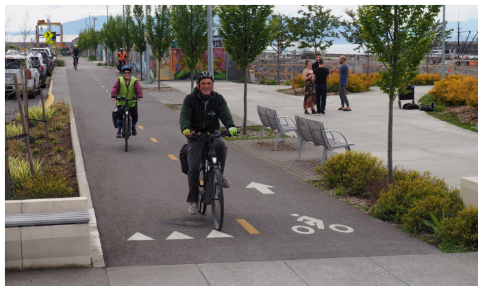
Separated Sidewalk Level, Two-Way Bicycle Lane on Granary Ave
