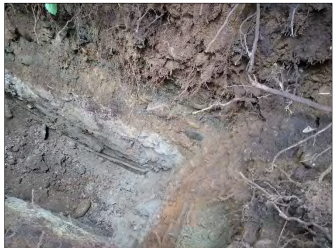
Photo 6: TP13; Thick Organic over Glacial Outwash and Dense Till
