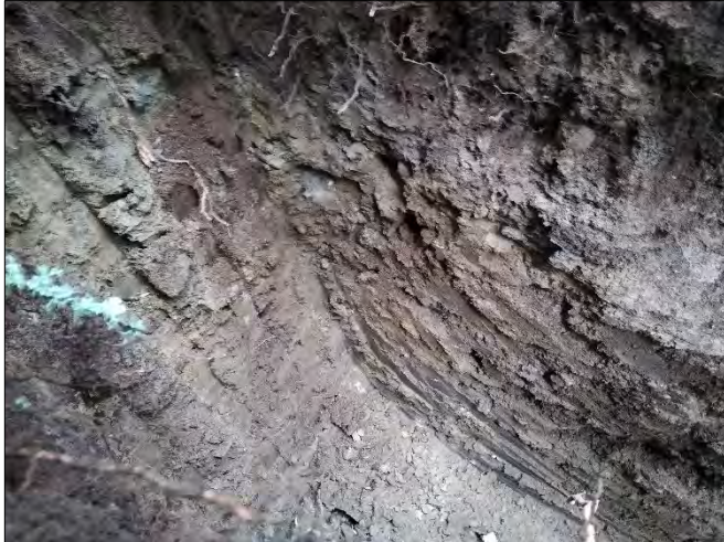
Photo 9: TP23; Glacial Drift over Dense Till
