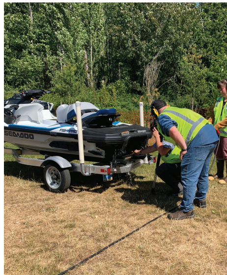
AIS program staff flushing the jet engine intake of a Personal Watercraft last used in Lake Mead, Nevada.
