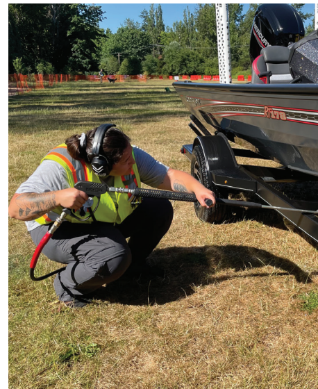
AIS program staff using hot, high-pressure water to decontaminate the hull and trailer of a watercraft.
