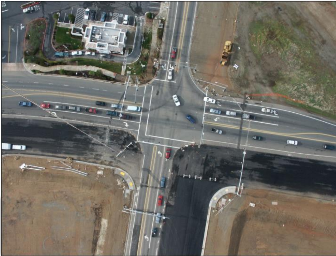
Intersection widening for vehicle capacity has made this a hostile place for walking and biking.
