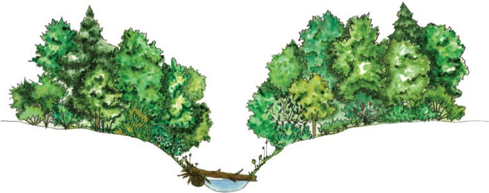
Typical existing to-be-retained channel section with additional vegetation and log structures, or created section where constraints preclude a wider floodplain.
