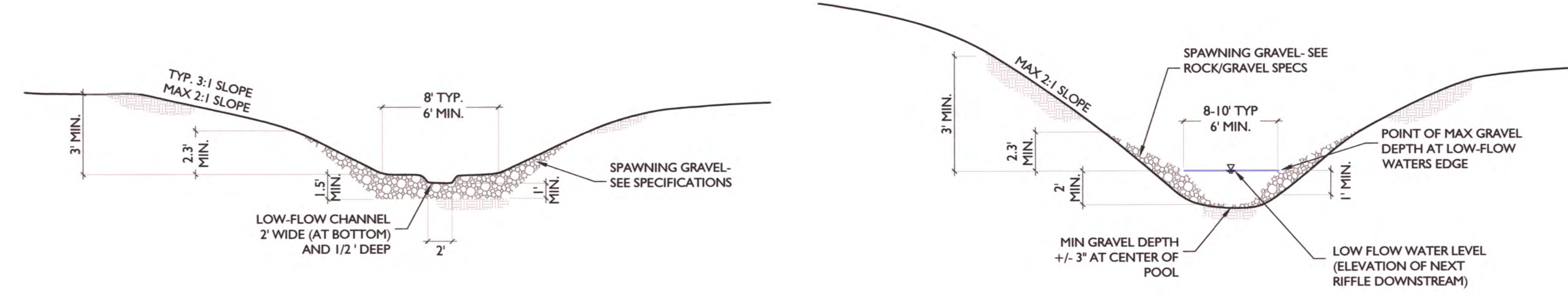
D TYPICAL RIFFLE CONSTRUCTION FOR REACH 3 NTS
