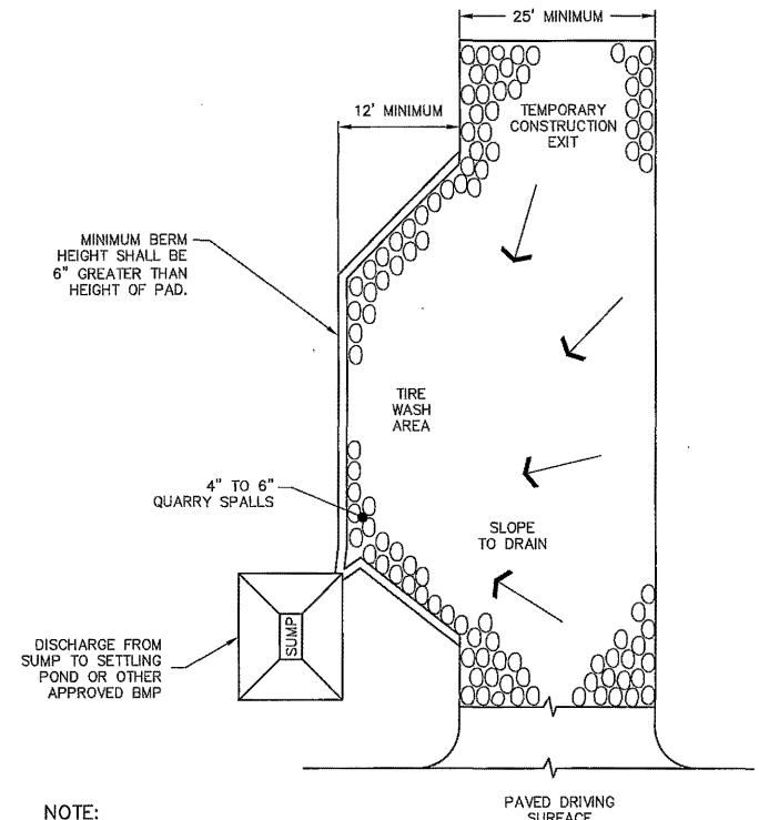
TIRE WASH AREA MUST BE INSTALLED DOWNGRADIENT OF TEMPORARY CONSTRUCTION EXIT. SURFACE
