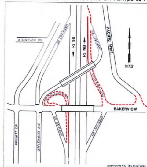
Exhibit PP2-E3: Alternative R-C: Combines new northbound and new southbound on-ramps to I-5
