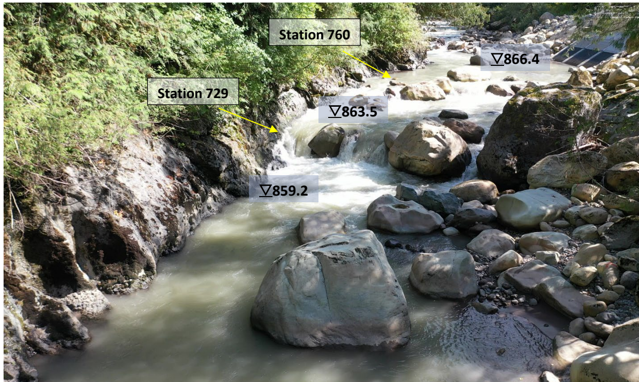
Figure 5.3 View of channel conditions between Station 663 (downstream photo extent) to the water intake structure upstream with water surface elevations extracted from the TLS scan on Sep. 12, 2022 at prominent channel steps (205 cfs).
