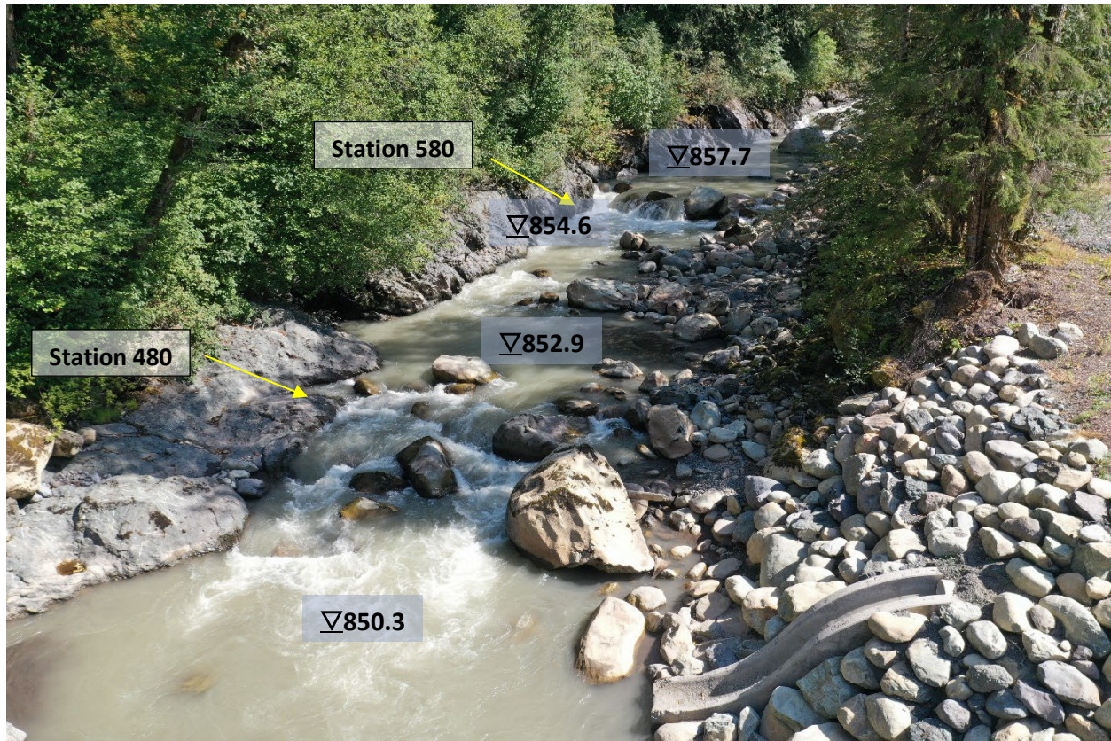
Figure 5.2 View of channel conditions between the fish outlet (Station 437) and Station 580 with water surface elevations extracted from the TLS scan on Sep. 12, 2022 at prominent channel steps (205 cfs).
