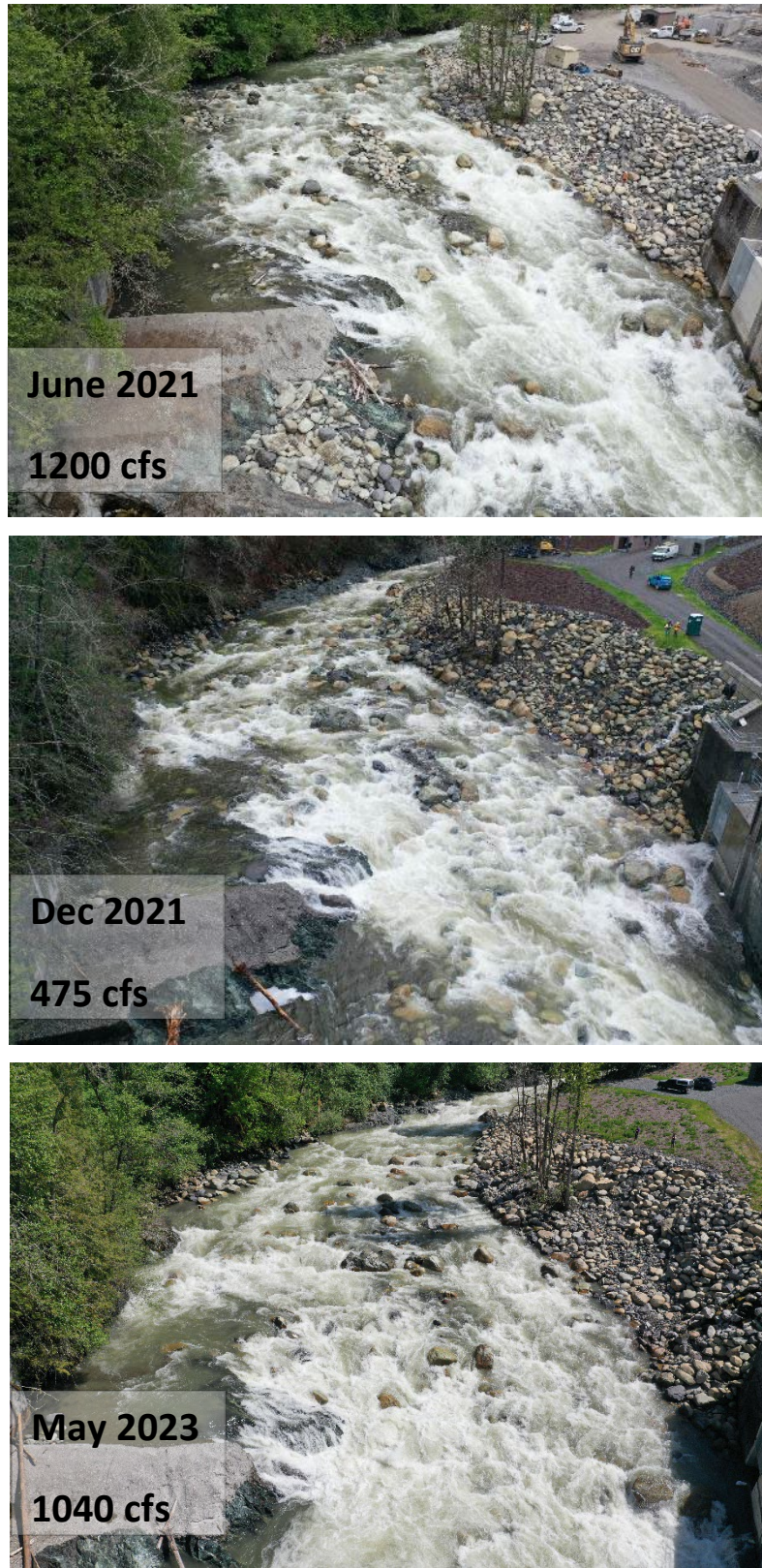
Figure 3.3 UAV oblique photos showing channel evolution at the flow split between the restored left bank channel and right bank pathways in June 2021 (top), December 2021 (middle), and May 2023 (bottom).
