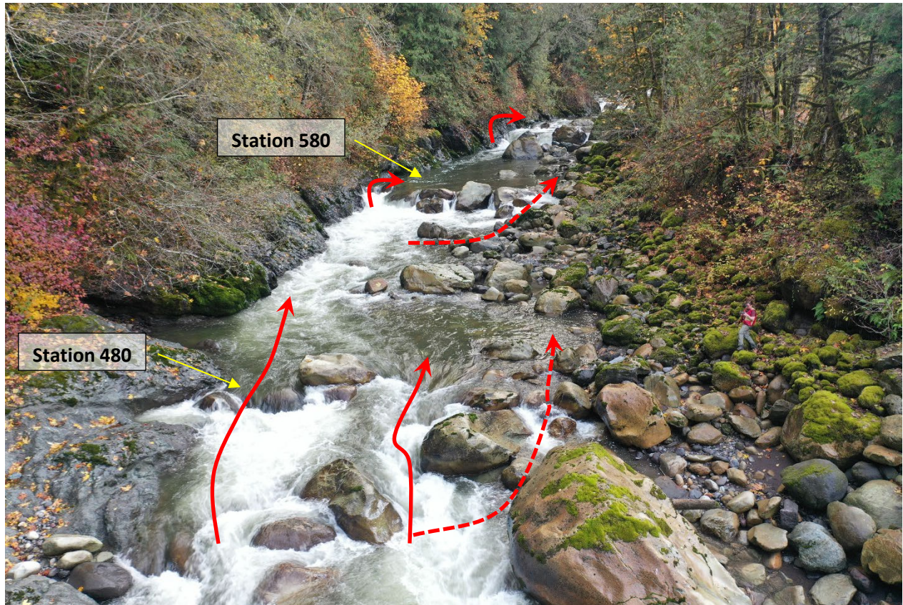
Figure 4.2 Likely passage routes at the observed flow at steps upstream of the fish outlet slide (October, 2025). Solid lines = expected primary pathway during lower to mid-flow range; dashed lines = additional routes during mid- and higher flow range.
