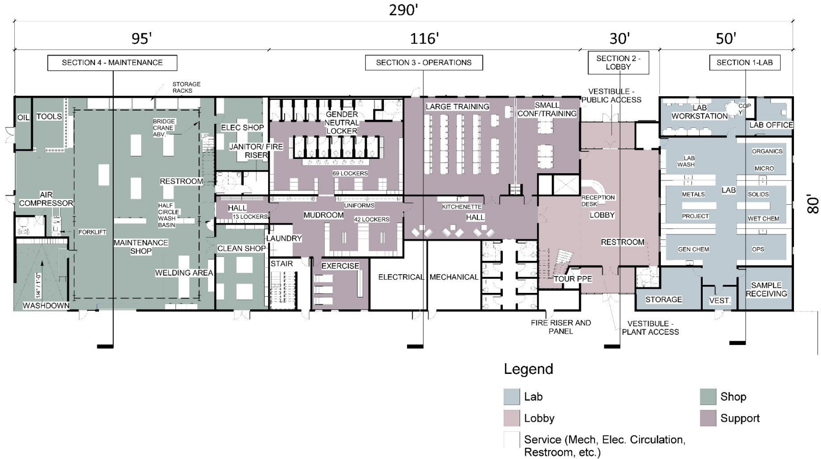
Figure 9-1. Revised Preferred Option First Floor Plan
