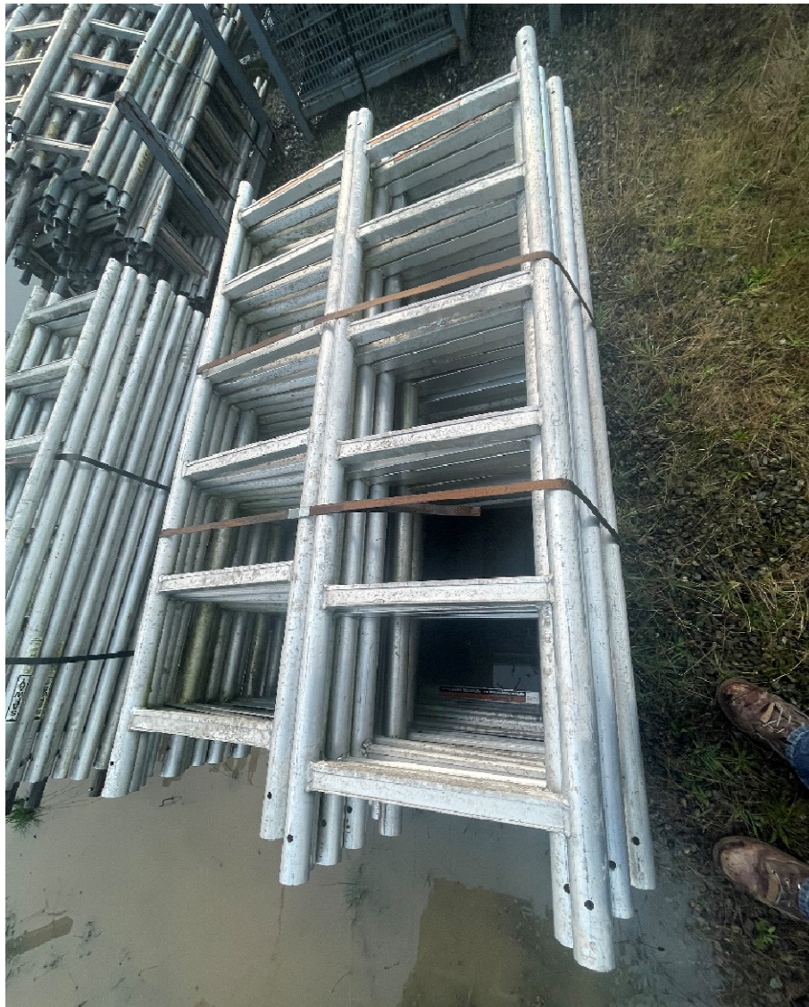
Figure 1: Segmented Ladder to Support Confined Space Entry
