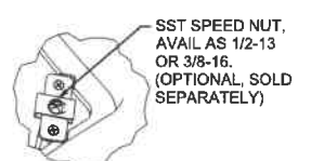
SST SPEED NUT, AVAIL AS 1/2-13 OR 3/8-16. (OPTIONAL, SOLD SEPARATELY) DETAIL F OPTIONAL SST SPEED NUT
