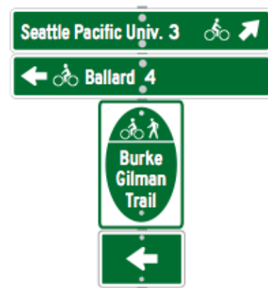
Decision and named route signs from Seattle. On trails, both sign types are used to mark the route and provide direction to destinations on and off the trail.
