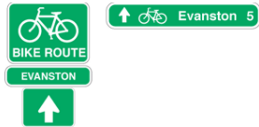
Above left: The D11-1 Bike Route sign. Above right: The D1-1c sign consolidates direction, destination and distance information onto one sign.
