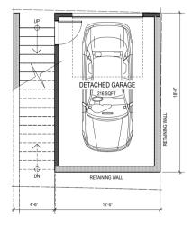
For a regular car space, City of Bellingham requires 18 feet minimum clear depth. The drawings illustrate a mid-size vehicle in the plans; a regular vehicle, such as a mini-van or truck, will not fit in this garage. Even with a mid-size vehicle, there is no allowance for recycling and garbage bin storage; thus, most would be placed in the driveway, forcing the second vehicle to park on the street, leaving no room for guests or pick-up and delivery services.
