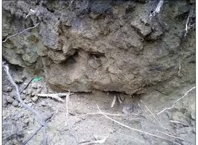
Photo 10: TP25; Sandy Eluvium Over Dense Sandstone Bedrock
