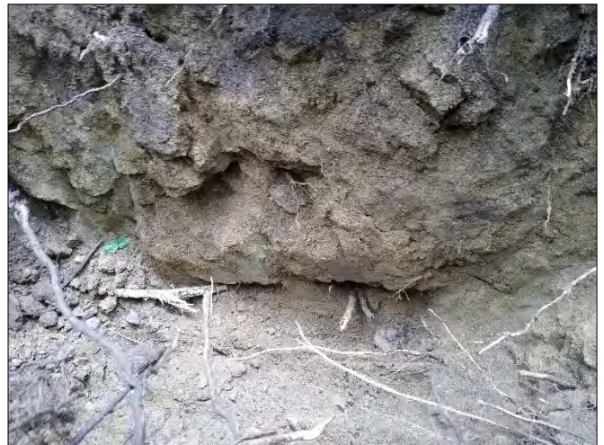
Photo 10: TP25; Sandy Eluvium Over Dense Sandstone Bedrock
