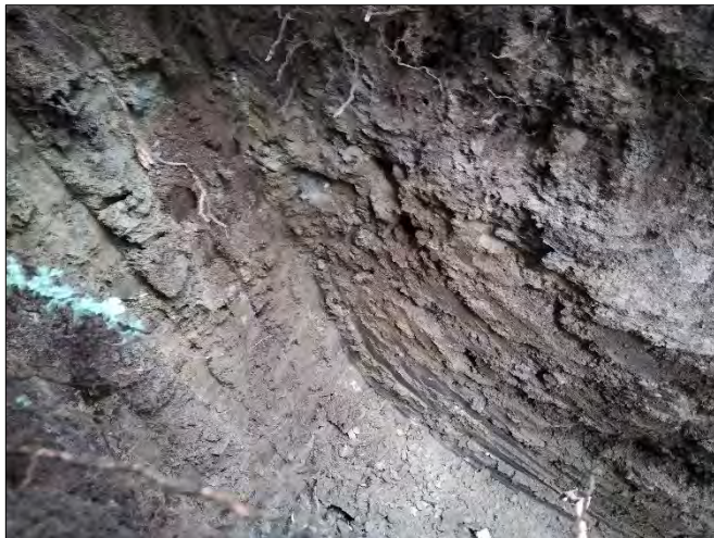
Photo 9: TP23; Glacial Drift over Dense Till
