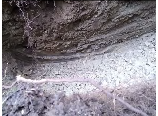
Photo 8: TP17; Dense Glacial Till at Base of Pit
