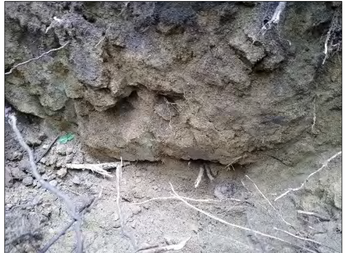
Photo 10: TP25; Sandy Eluvium Over Dense Sandstone Bedrock
