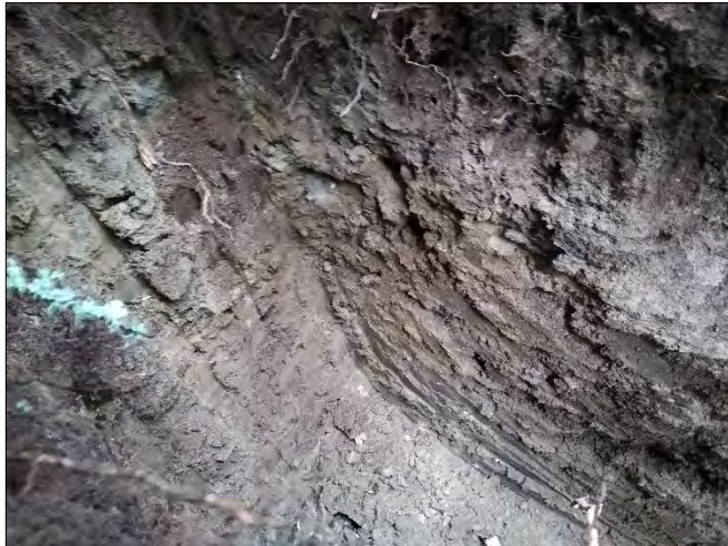
Photo 9: TP23; Glacial Drift over Dense Till
