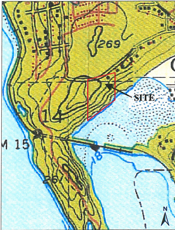
FIGURE 2: The geology of the site is mapped as Chuckanut Formation (TKc) (Easterbrook 1976). Numerous outcrops of sandstone were at the site. The more resistant and massive beds often form substantial cliffs throughout the site. Bedding strike was roughly N80E (260 degrees) and dipped to the north at approximately 40 degrees. The site is located near or within the hinge of a large anticline that plunges to the northwest (See Figure 3).
