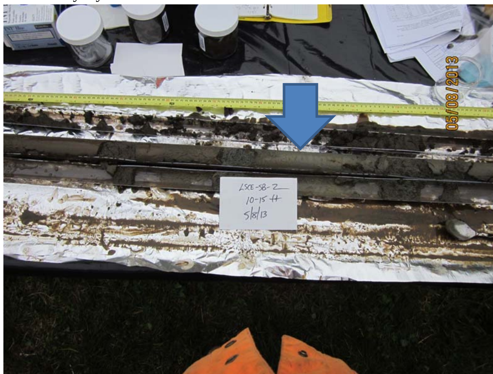
Photograph 6. Soil core from LSCE-SB-2 (10-15 ft depth), note the ~1 ft clay layer above sand layer.
