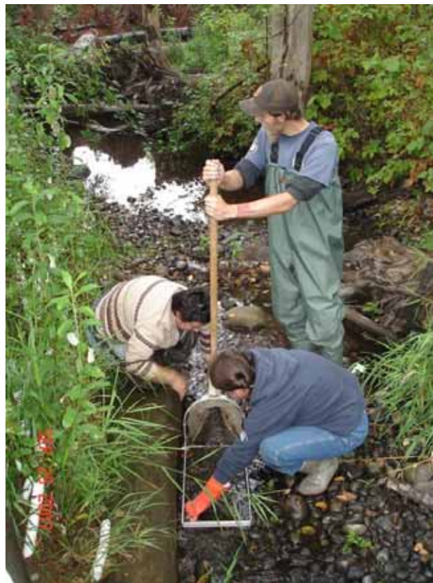
Figure 2-13. WCC staff collecting a macroinvertebrate sample using the D-frame kick net.
