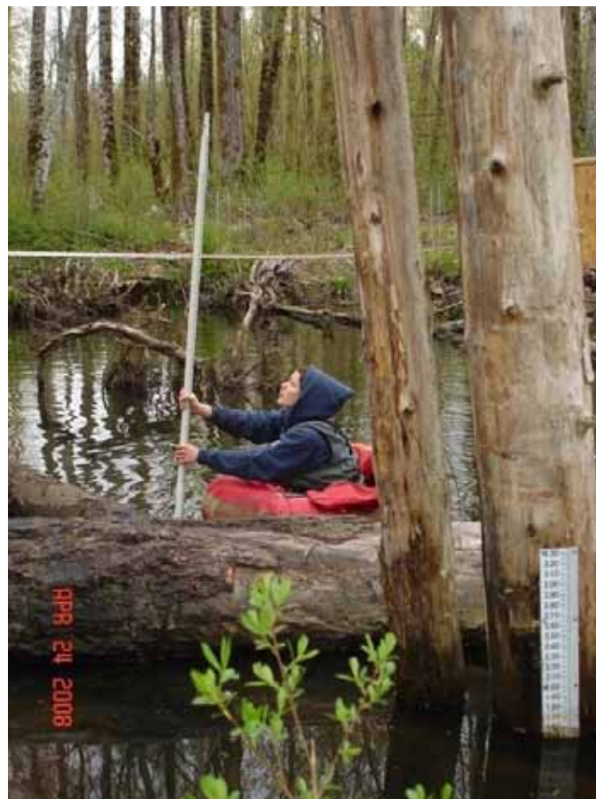
Figure 3-3. WCC surveyor using stadia rod to measure pond depth along transect marked by measuring tape, April 24, 2008. Staff gage in foreground.
